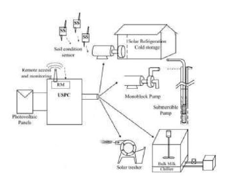
Fig. 1. USPC operation schematic diagram.
